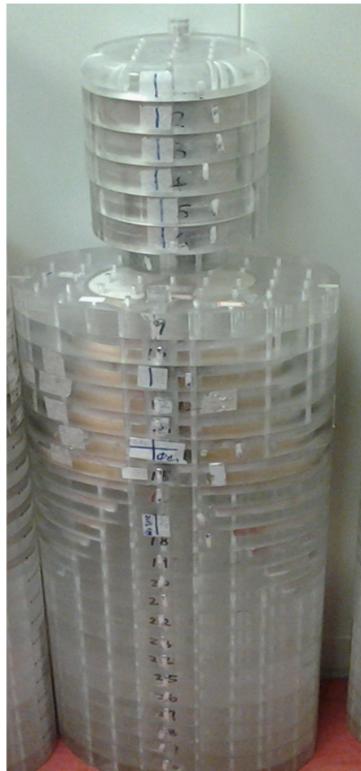
Figure 4: 70 kg Phantom with marked TLD measurement positions.
